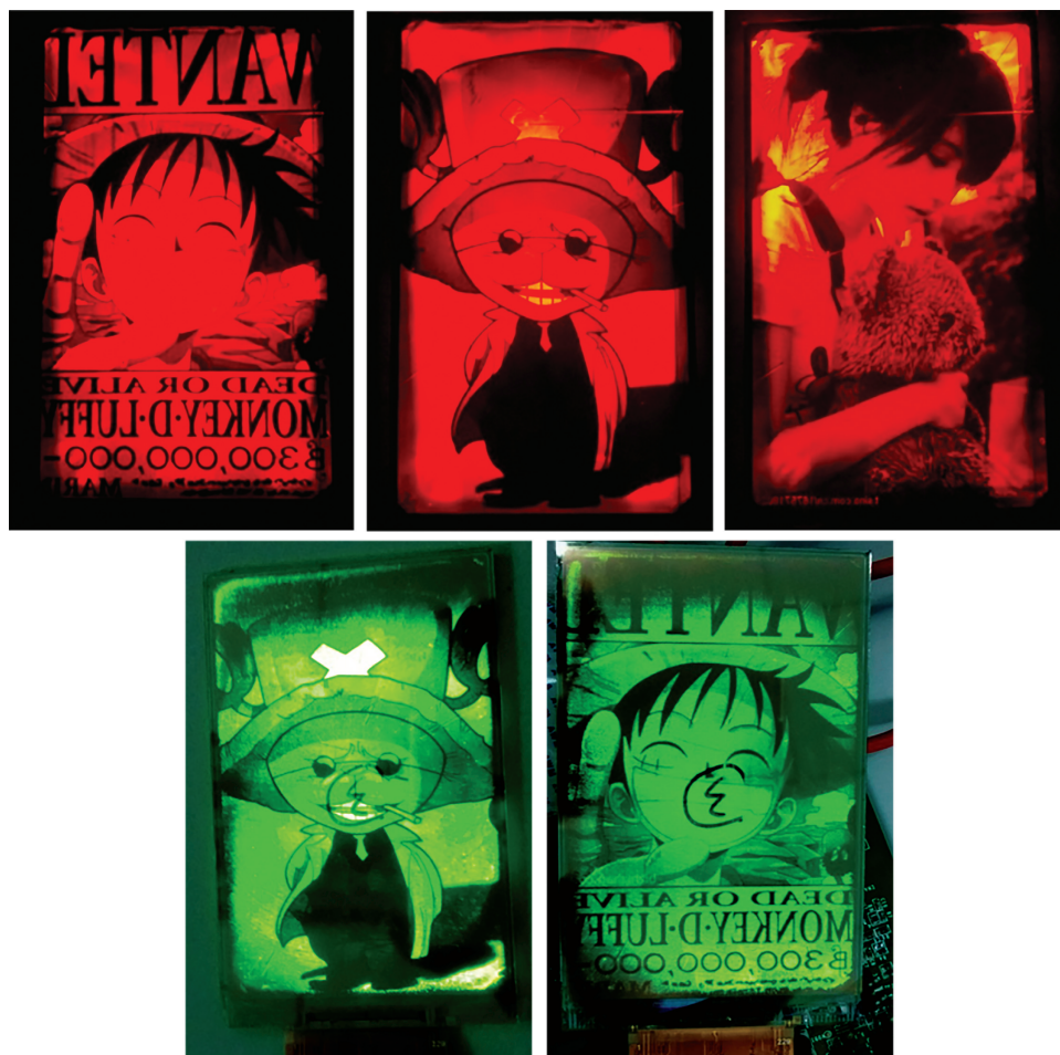
Figure 5 | Monochrome active matrix QD-LED display prototypes. Electroluminescence images of the 4.3-inch red and green active matrix QD-LED display prototypes with a resolution of 480 \times 800 using an LTPS TFT backplane.
