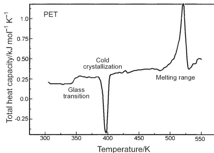
**Fig. 2** Total heat capacity of PET deconvoluted from a run as given in Fig. 1a from 315 to 555 K (240 sawtooth modulation cycles)
