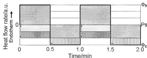
**Fig. 1c** Schematic drawing of the thermal response as in Fig. 1b, but with the addition of an irreversible, exothermic latent heat represented by the vertically shaded areas (non-linear but stationary)
