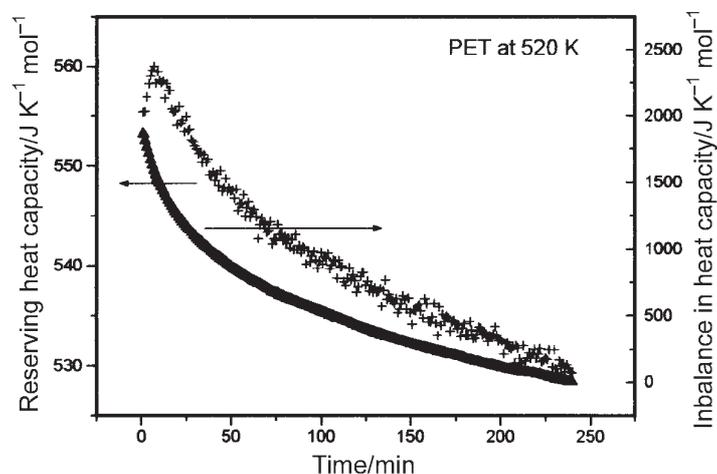
**Fig. 5** Reversing heat capacities (crosses) and the imbalance in heat capacities (triangles) of PET during a quasi-isothermal measurement at 520 K, using the quasi-isothermal analysis under conditions as in Fig. 4
