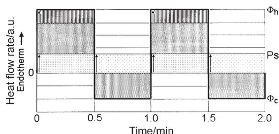
**Fig. 1e** Schematic drawing of the thermal response as in Fig. 1b, but with the addition of an irreversible, endothermic latent heat during the first half of each cycle as represented by the vertically shaded areas (non-linear and non-stationary)
