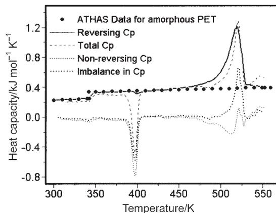
**Fig. 3** Analysis of the data from Fig. 2 with the standard DSC method. Reversing heat capacity from Eq. (4), total heat capacity from Eq. (1) with the total heat-flow rate and underlying heating rate, non-reversing heat capacity from the difference between reversing and total heat capacity, and imbalance of heat capacity from Eq. (5). Also listed are the data bank data for the heat capacity of amorphous PET
