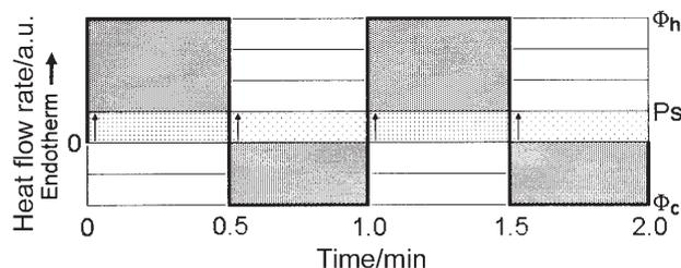
**Fig. 1b** Schematic drawing of the linear thermal response (solid lines) for the temperature program of Fig. 1a. The effects of the underlying (lightly dotted boxes) and reversing responses (heavily dotted boxes) are indicated. The heavy line represents  $\Phi(t)$ , and the pseudo-isothermal level ( $Ps$ ), the zero level and the value of  $\Phi_h$  and  $\Phi_c$  are marked
