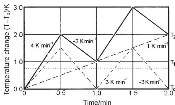
**Fig. 1a** Schematic drawing of sawtooth-type modulation (solid line) and its deconvoluted underlying heating rate  $\langle \dot{T} \rangle$  and reversing rate of temperature change of  $\pm 3 \text{ K min}^{-1}$  (dashed lines). The temperatures listed on the right indicate the beginnings and ends of the cycles
