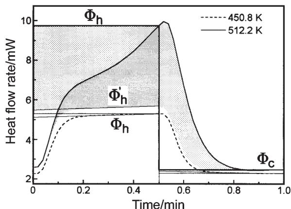
**Fig. 6** Baseline-subtracted heat-flow rates of PET for a single sawtooth at 450 and 512 K from the experiment of Fig. 2
