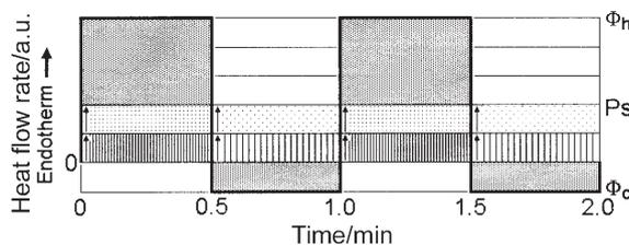
**Fig. 1d** Schematic drawing of the thermal response as in Fig. 1b, but with the addition of an irreversible, endothermic latent heat represented by the vertically shaded areas (non-linear but stationary)
